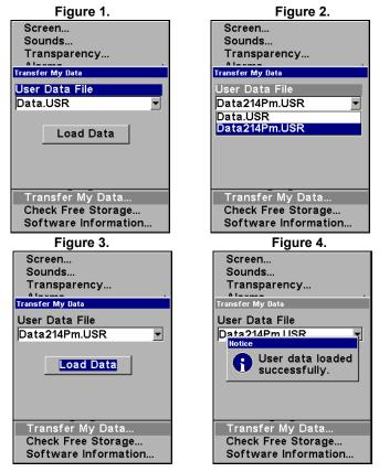
These figures show the menu sequence for loading a GPS Data File from an MMC into the unit's memory.
